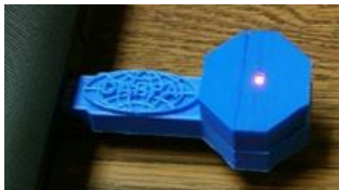
Figure 12 Fully 3D printed lighted LED dongle
