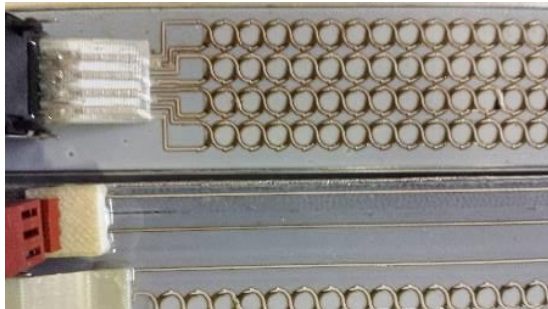
Figure 6 3D printed twisted pair connection to RJ-45 jack
