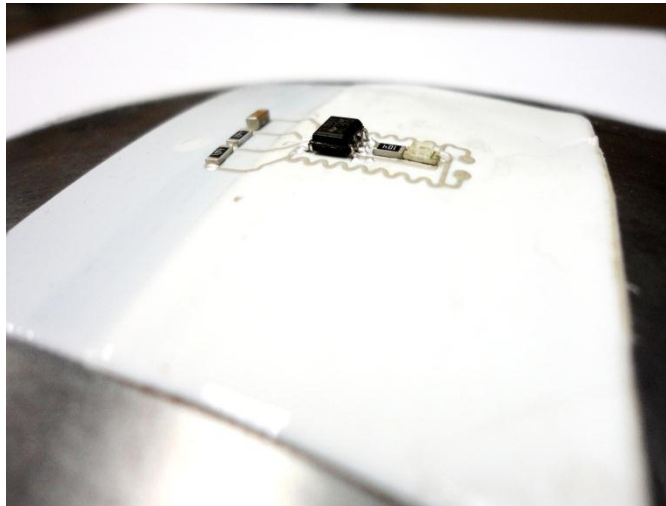
Figure 14 - Completed test circuits built with DPAM process. The left photo is on a flat surface, the right photo is a curved surface.
